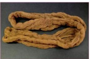
(Left) Schematic illustration of the process of preparing conductive cotton yarns via in-situ free radical polymerization (Only grafting of PMANa is illustrated here. Grafting of PAANa follows the same procedures). (Right) As-made PMANa-assisted copper-coated cotton yarns. Credit: Hong Kong PolyU
