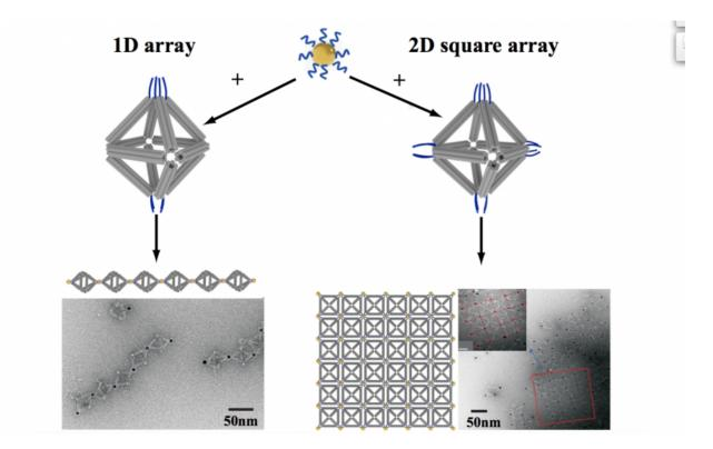
By strategically placing tethers on particular vertices, the scientists used the octahedrons to link nanoparticles into one-dimensional chainlike arrays (left) and two-dimensional square sheets (right). Credit: Brookhaven National Laboratory
