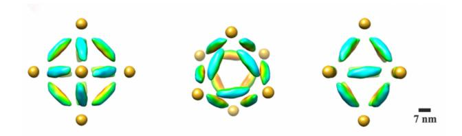
A combination cryo-electron microscopy image of an octahedral frame with one gold nanoparticle bound to each of the six vertices, shown from three different angles. Credit: Brookhaven National Laboratory
