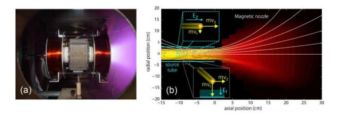
(a) Photograph of the helicon plasma thruster at Tohoku University. (b) The measured plasma pressure profile and the particle dynamics relating to the loss of axial momentum loss. Credit: Kazunori Takahashi
