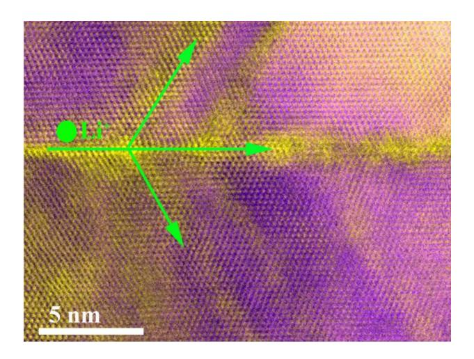
Spotting twin boundary defects in tin oxides requires the aid of a transmission electron microscope: The yellow streaks, highlighted by green arrows, show where lithium ions travel along twin boundaries. Credit: Reza Shahbazian-Yassar
