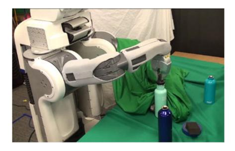
BRETT is shown here learning how to screw a cap onto a water bottle. Credit: UC Berkeley Robot Learning Lab
