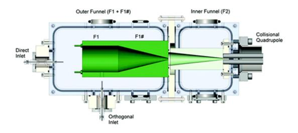
The high-flux soft landing instrument incorporates two ion funnels, with a larger funnel feeding into a smaller one, to achieve an ion deposition rate of 1 microgram per day, significantly faster than previous approaches. This technique creates mesoscale structures that were not feasible before, answering questions that are key in energy production, conversion, and storage. Credit: Gunaratne et al. 2015 with permission from The Royal Society of Chemistry.
