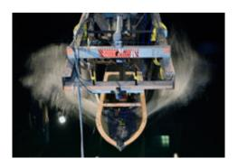
Earlier this month, scientists sponsored by the Office of Naval Research (ONR) performed experiments to better understand the motions, forces and pressures generated by waves on boats with high-speed planing hulls.
