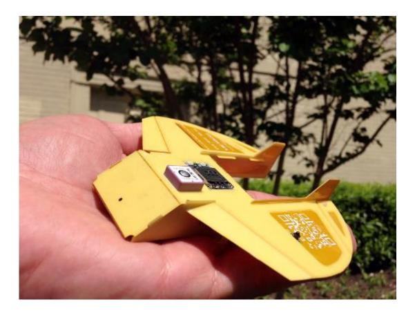
The Cicada drone can fly at about 46 miles (74 kilometers) per hour and are virtually silent, with no engine or propulsion system
