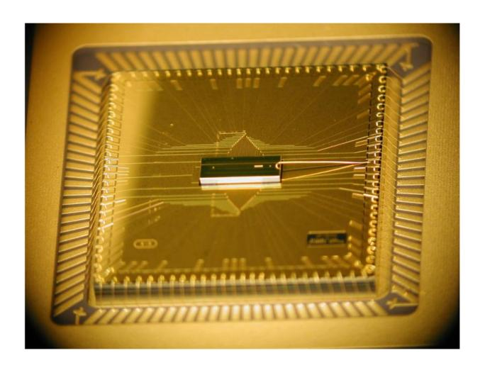
A photograph of the completed BGA trap assembly. The trap chip is at the center, sitting atop the larger interposer chip that fans out the wiring. The trap chip surface area is 1mm x 3mm, while the interposer is roughly 1 cm square. Credit: D. Youngner, Honeywell
