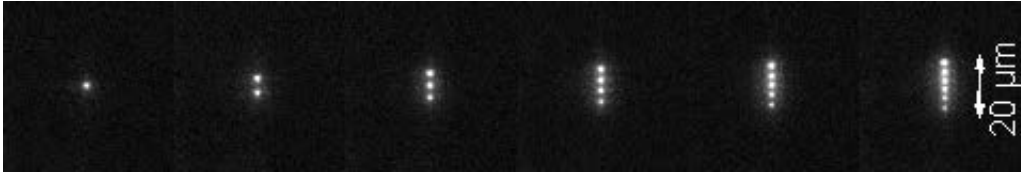
Fluorescence images of calcium ions confined in the BGA trap. Credit: N. Guise, GTRI
