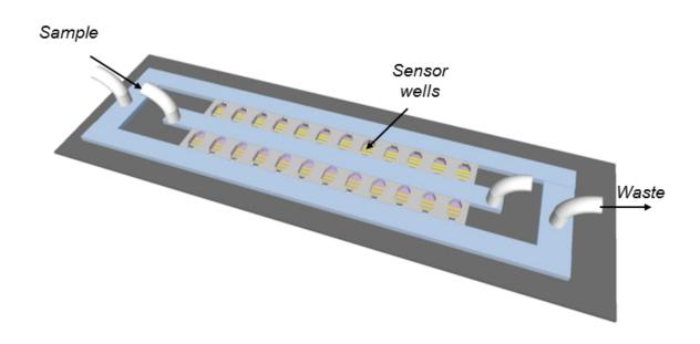
Schematic of the antibiotic susceptibility testing device. The bacteria are cultured in miniature chambers, each of which contains a filter for bacterial capture and electrodes for readout of bacterial metabolism Credit: University of Toronto
