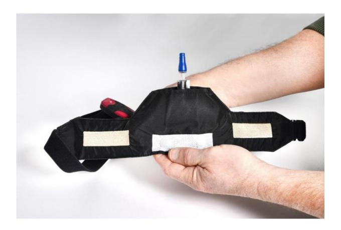
The prototype chest strap ECG-monitor has been tested in over hundred experiments on male and female subjects. Credit: Empa
