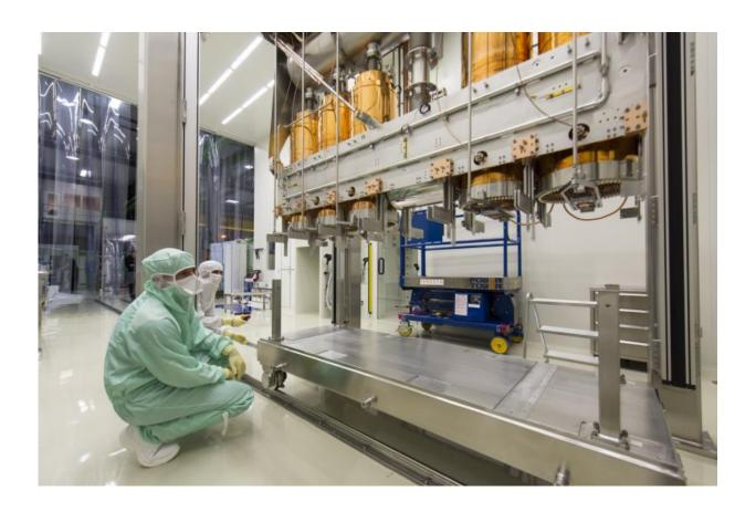
The first HIE-ISOLDE acceleration module was assembled over the last few months in a new clean room. Credit: Maximilien Brice/CERN
