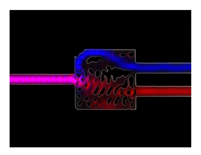
Infrared light enters this silicon structure from the left. The cut-out patterns, determined by an algorithm, route two different frequencies of this light into the pathways on the right. This is a greatly magnified image of a working device that is about the size of a speck of dust. Credit: Alexander Piggott
