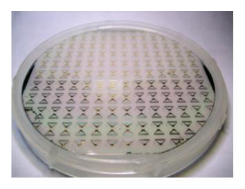
A photograph of a four-inch piezoelectric wafer containing fabricated sensors. Credit: A\*STAR Institute of Materials Research and Engineering
