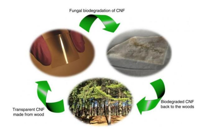
An illustration of a likely life cycle of the biobased and biodegradable CNF paper. First, cellulose nanofibrils (CNFs) extracted from the woods is made into CNF paper. The CNF paper can be degraded via fungal biodegradation and sent back to the woods without adverse environmental effects. Credit: University of Wisconsin-Madison
