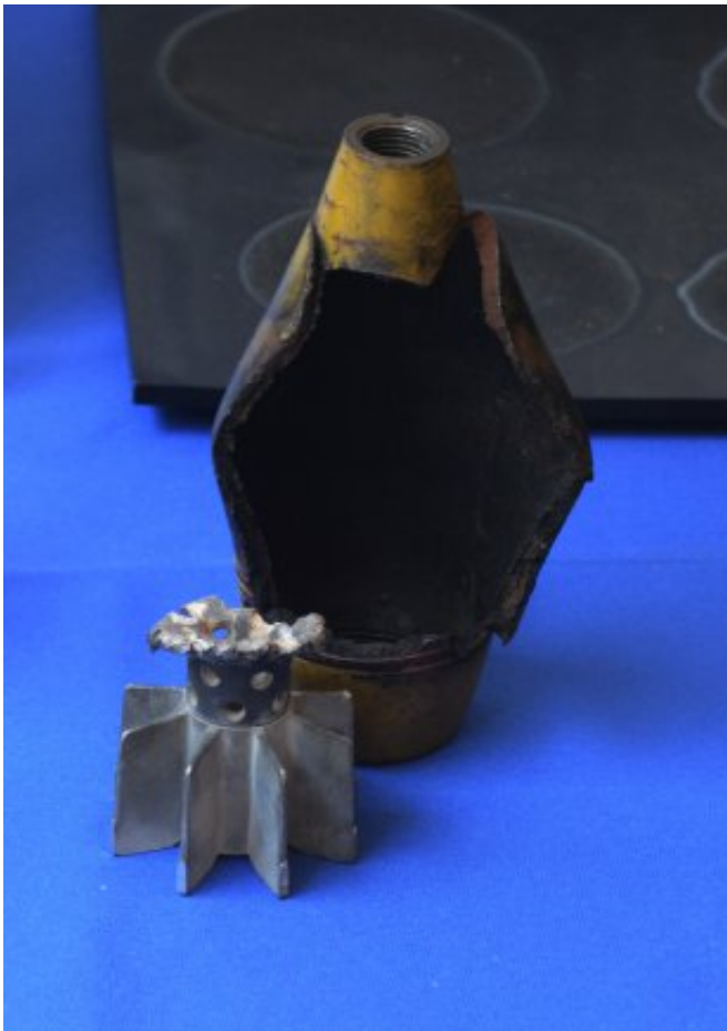
A 60-mm mortar round fried open by a High Energy Laser Mobile Demonstrator
