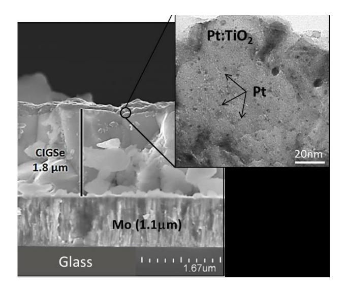
A scanning electron microscopy shows a cross section of the composite photocathode (left). By TEM analysis, nanoparticles of Pt could be identified in the TiO2 thin film (right). Credit: HZB
