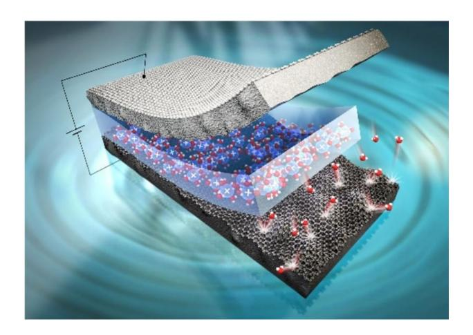
Schematic of the ionic polymer-graphene composite (IPGC) actuator or "motor". When an electric field is applied, the redistribution of ions causes the structure to bend. Credit: Korea Advanced Institute of Science and Technology
