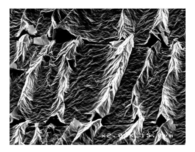
Researchers from Brown University have developed new graphene surfaces, engineered with tiny wrinkles, as environments for cell culture. The surfaces could provide a way to culture cells in the lab that better approximates the complex environments in which cells grow in the body. Credit: Hurt Lab/Brown University
