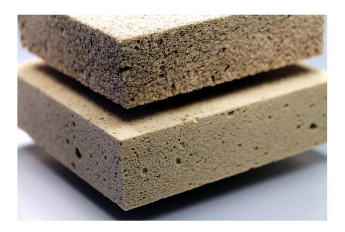
These rigid foam insulation boards are 100% wood-based. Credit: © Manuela Lingnau / Fraunhofer WKI
