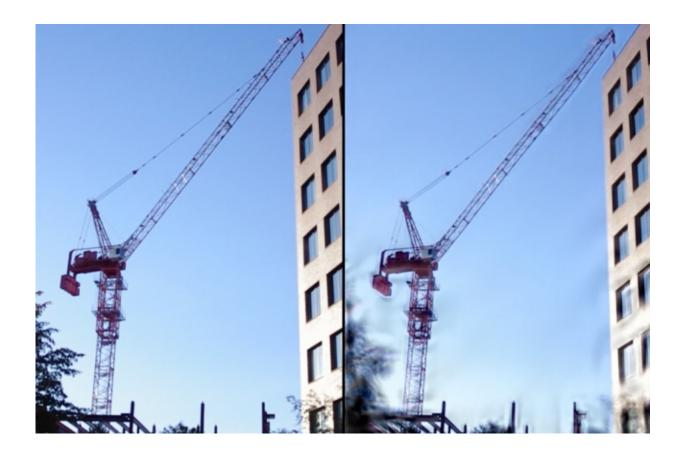
Motion magnification of a crane imperceptibly swaying in the wind. The source video is on the left, and the motion magnified video is on the right, with magnification of 100 times greater in the frequency band of 0.2 Hz to 0.25 Hz.
