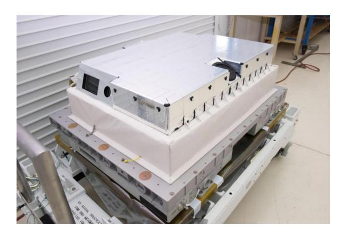
The completed flight assembly of the High Definition Earth Viewing unit before it was launched to the International Space Station in 2014. Credit: NASA
