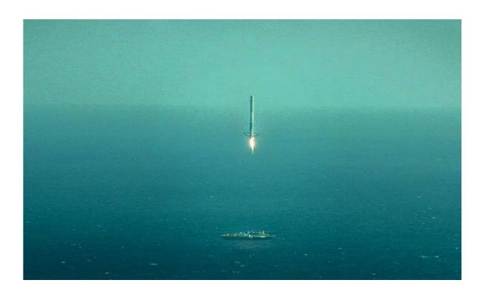
View of Falcon 9 first stage landing burn and touchdown on 'Just Read the Instructions' landing barge. Credit SpaceX
