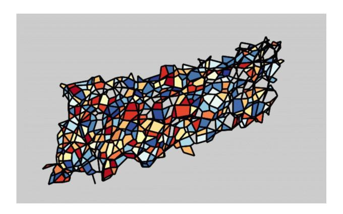
This theoretical representation of experimental data (Behringer Lab.) provides a quantitative tool for identifying the fluid to solid transition in a granular solid. The fluctuations in the net show the change in strength of the solid. Credit: Sumantra Sarkar, Brandeis University
