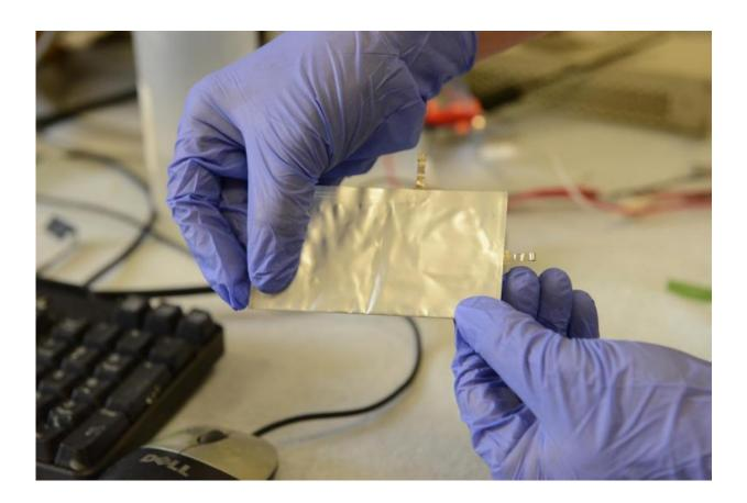
Stanford scientists have invented a flexible, high-performance aluminum battery that charges in about 1 minute. Credit: Mark Shwartz, Precourt Institute for Energy, Stanford University
