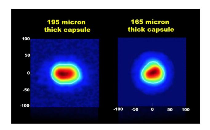
X-ray images from recent National Ignition Facility implosion experiments compare two shots with different thickness ablators, demonstrating the improvement in shape. Both shots used deuterium-tritium fuel and were fired at 350 terawatts of ultraviolet laser power.
