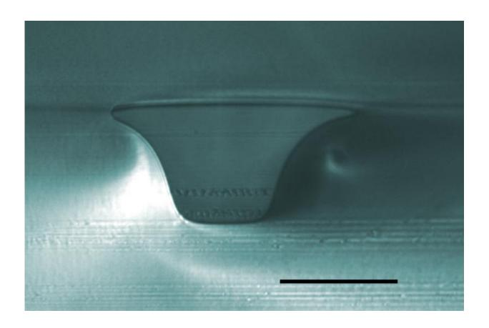
NIST found a combination of techniques to effectively measure microfluidic channels, achieving an accuracy of within 5 percent for both a channel's depth and its bottom's width. Scale bar in this cross-section of a channel represents 50 micrometers. Credit: Reyes/NIST
