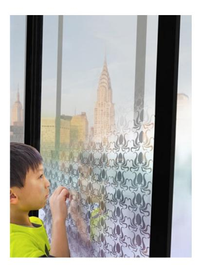
This illustration shows how a full-sized "smart" window could switch from transparent to an opaque pattern, via a motorized stretcher hidden in the frame. Credit: Jenny Sabin
