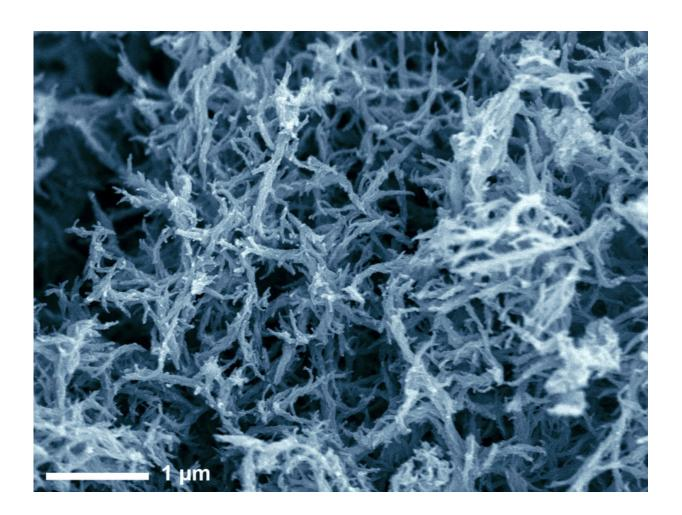
A recipe for nanofibres: Scientists at the Max Planck Institute of Colloids and Interfaces produce spherical, sheet-like and fibrous nanostructures by carbonising various organic solvents in hot salt melts. Until now, it was only possible to carbonise solids, resulting in spherical particles. Credit: MPI of Colloids and Interfaces
