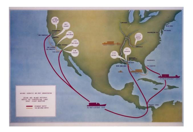
The illustration above shows routes on which barges transported pieces of the Saturn V rocket to and from test facilities and the launch site in the mid to late 1960s. Credit: NASA's Marshall Space Flight Center
