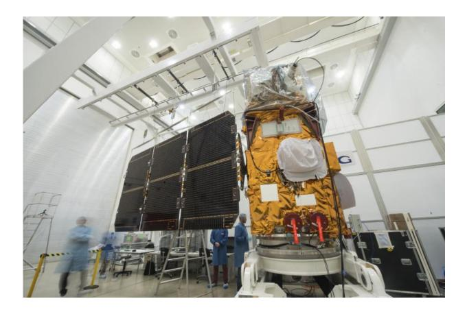
The final solar wing deployment test marks the end of a six-month programme at IABG in Germany to make sure the satellite can withstand the shocks and vibrations during liftoff and that it is fit for a long working life in the harsh environment of space. The next step is to pack up the satellite in its container and ship it to Europe's Spaceport in French Guiana for launch, which is scheduled for 12 June 2015. Credit: ESA/M. Pedoussaut
