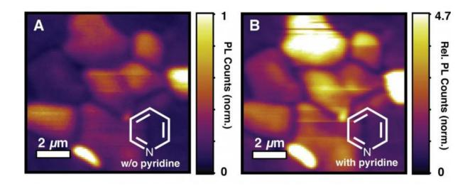
The quality of the perovskite materials for electronic device applications improved after chemical treatment, remediating the "dark" areas. Credit: University of Washington
