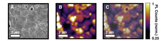
UW researchers used microscopy to identify inefficient regions in perovskite materials used in solar cells, as evidenced by dark areas in C. Credit: University of Washington
