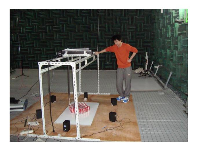
Coauthor Gen Gu of Nanjing University with the soda can array in the anechoic (non-echoing) room. Although the array achieves extraordinary acoustic focusing due to its metamaterial properties, the scientists found that it does not truly beat the diffraction limit. Credit: A. A. Maznev, et al.
