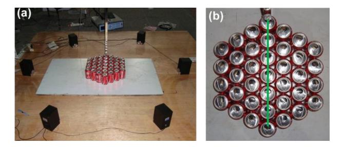
Experimental arrangement of the soda can array inside the anechoic room. The green line shows the scan line of the microphone that measures the acoustic intensity of the array. Credit: A. A. Maznev, et al. CC-BY-3.0
