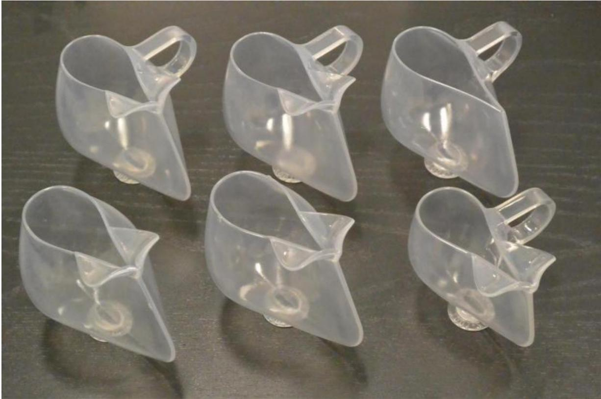
The ISSpresso technology demonstration will employ a cup specially designed to conduct the Capillary Beverage investigation for fluid physics aboard the International Space Station. Credit: Andrew Wollman
