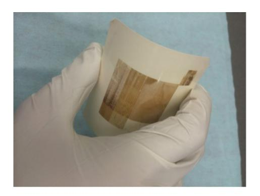
A high-mobility polysilicon layer was directly formed on paper by coating liquid silicon, which was annealed by pulsed laser-light. Credit: R. Ishihara, M. Trifunovic/TUDelft
