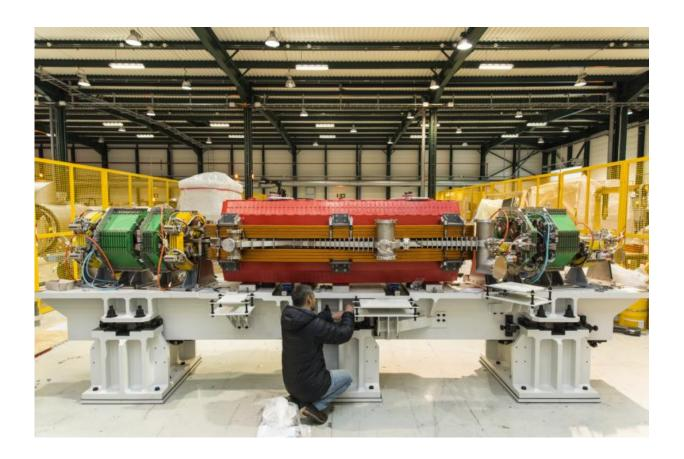
An engineer tests the installation of a vacuum chamber for SESAME, at CERN's magnet-testing facility SM18. Credit: Maximilien Brice/CERN
