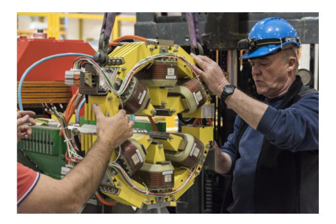
Engineers test the installation of a vacuum chamber for SESAME at the CERN magnet-testing facility SM18. Credit: Maximilien Brice/CERN
