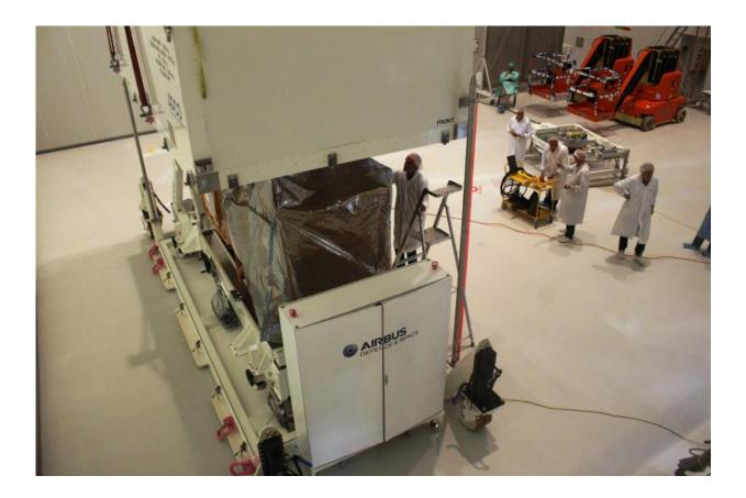
The Sentinel-2A container in the cleanroom at Europe's Spaceport in Kourou, French Guiana. Engineers use a crane to open the container that protected the satellite during its voyage from Munich in Germany. The satellite will spend the coming weeks beginning prepared for launch on 11 June 2015. Credit: ESA–C. Wildner
