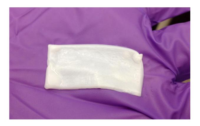
Pictured is an image of engineered collagen tissue matrix created in the laboratory of Sherry Harbin, Purdue associate professor of biomedical engineering. The engineered collagen polymer "looks like tissue, handles like tissue, and performs like tissue." Since this engineered tissue matrix is designed at the molecular level, it can be customized in terms of geometry, fibril microstructure, mechanical properties and cell-instructive capacity. Credit: Sherry Harbin
