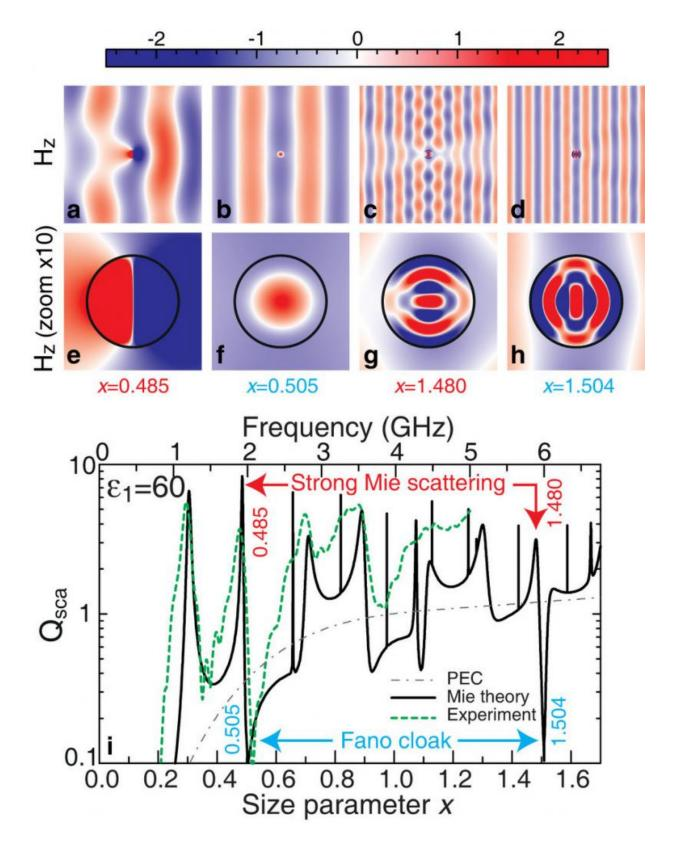
Scattering calculations from a single cylinder filled with water. Shown are:
