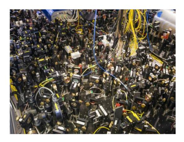
Growing artificial crystals: In this jumble of optical instruments, researchers from the Max Planck Institute of Quantum Optics use laser beams to create an optical lattice in which they trap rubidium atoms. Using a further laser, they excite a few of the atoms to become Rydberg atoms, which then form a magnetic quantum crystal. Credit: Axel Griesch
