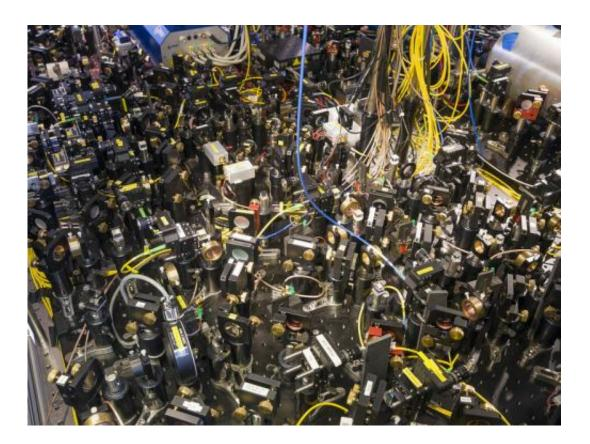
Growing artificial crystals: In this jumble of optical instruments, researchers from the Max Planck Institute of Quantum Optics use laser beams to create an optical lattice in which they trap rubidium atoms. Using a further laser, they excite a few of the atoms to become Rydberg atoms, which then form a magnetic quantum crystal. Credit: Axel Griesch
