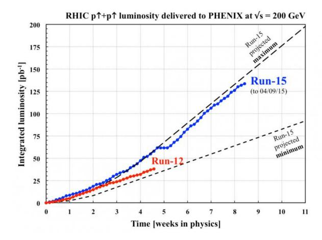
RHIC is producing more than twice as many proton-proton collisions per week during the current run as it did in 2012, the last run dedicated to polarized proton collisions. Credit: Brookhaven National Laboratory
