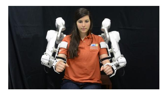
Researchers in the Cockrell School of Engineering at The University of Texas at Austin have developed a first-of-its kind, two-armed, robotic rehabilitation exoskeleton that could provide a new method of highquality, data-driven therapy to patients suffering from spinal and neurological injuries.
