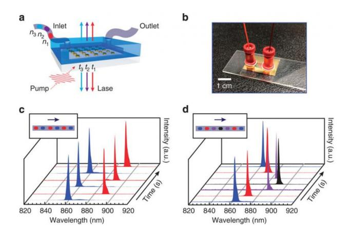
Lasing emissions from Au NP arrays tuned in real time. Credit: *Nature Communications* 6, Article number: 6939 doi:10.1038/ncomms7939
