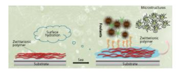
The block copolymer alters its structure in response to salt solution, enabling it to survive intact in dynamic marine environments. The material may prove useful for creating non-toxic alternatives to antifouling paint used on boats. Credit: A\*STAR Institute of Chemical and Engineering Sciences
