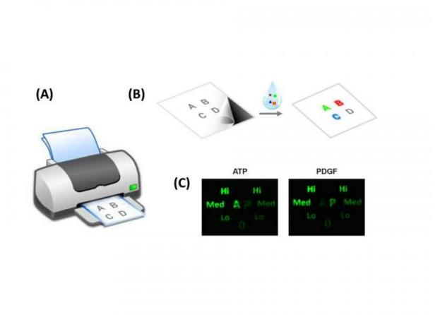
A) Making paper sensors using a regular irkjet printer with cartridge containing DNA-based bio-irk. B) The paper sensor is simple to use - add a droplet of test sample and look for the right text to show up. (C) A real sensor designed to detect two biomarkers, ATP ( a small-molecule biomarker for abcteria) and PDGF (a protein biomarker for cancer). 'A' lights up when ATP is present and 'P' lights up when the test sample has PDGF. Credit: McMaster University
