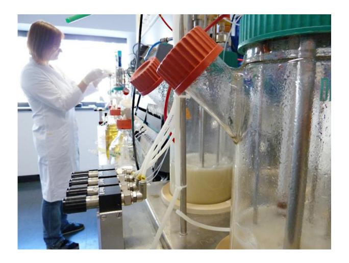
acib researcher Tamara Wriessnegger is manipulating a bioreactor with yeast producing valuable nootkatone. Credit: acib
