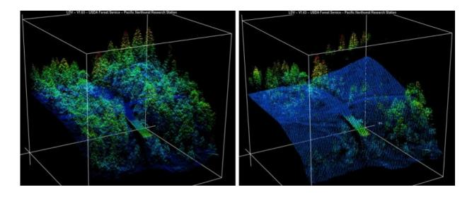
These before-and-after lidar images from the King fire show an area on the west side of the Rubicon River where fire damage was severe. Blue is ground level; lighter colors are higher. A road, bordered by dense trees in the before image, and part of a bridge (green) are at center. Credit: USFS
