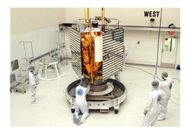
In this undated photo provided by NASA, technicians with The Johns Hopkins University Applied Physics Laboratory in Titusville, Fla., prepare the MESSESNGER spacecraft for a move to a hazardous processing facility in preparation for loading the spacecraft's hypergolic propellants. (NASA via AP)
