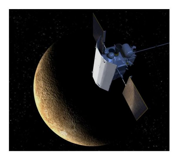
This artist's rendering provided by the Johns Hopkins University Applied Physics Laboratory shows the sunshade on the MErcury Surface, Space ENvironment, GEochemistry, and Ranging (Messenger) around the planet Mercury. The sunshade shields the spacecraft's instruments from heat and solar radiation. (Johns Hopkins University Applied Physics Laboratory via AP) Image converted using ifftoany
