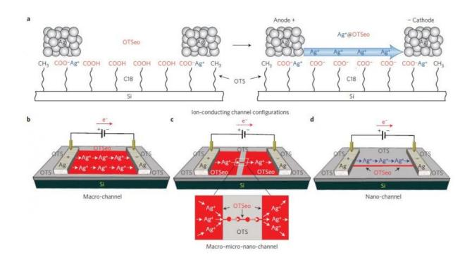
Schematic representation (not to scale) of proposed bias-driven ionic transport in the dilerent ion-conducting pattern configurations investigated in this study. Credit: (c) *Nature Materials*, doi: 10.1038/nmat4254
