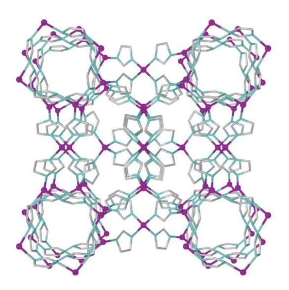
Filigree cages: Using a variant of powder X-ray diffraction co-developed by scientists at the Max Planck Institute for Solid State Research, an international team has discovered a previously unknown structure of the metal-organic framework compound ZIF-8. The researchers named the new structure katsenite.
