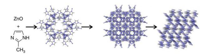
Structural transformation in the mill: The katsenite structure exists in two variants shown by the two structures to the right. They form during the mechanosynthesis of ZIF-8 from solid starting substances (left) in a ball mill. During the reaction, the familiar structure of ZIF-8 emerges. Mechanosyntheses can now be monitored in real-time with the help of a modified X-ray diffraction method. This could shed light on approaches for optimising such processes. Credit: Nature Communications
